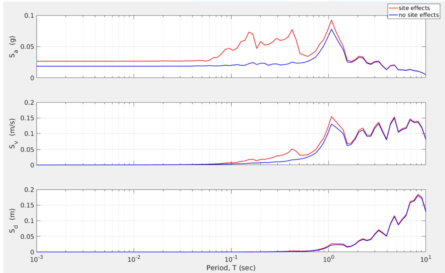
■ Hypocentre in the middle of the fault      ■ Mw = 8.1      ■ NS component
