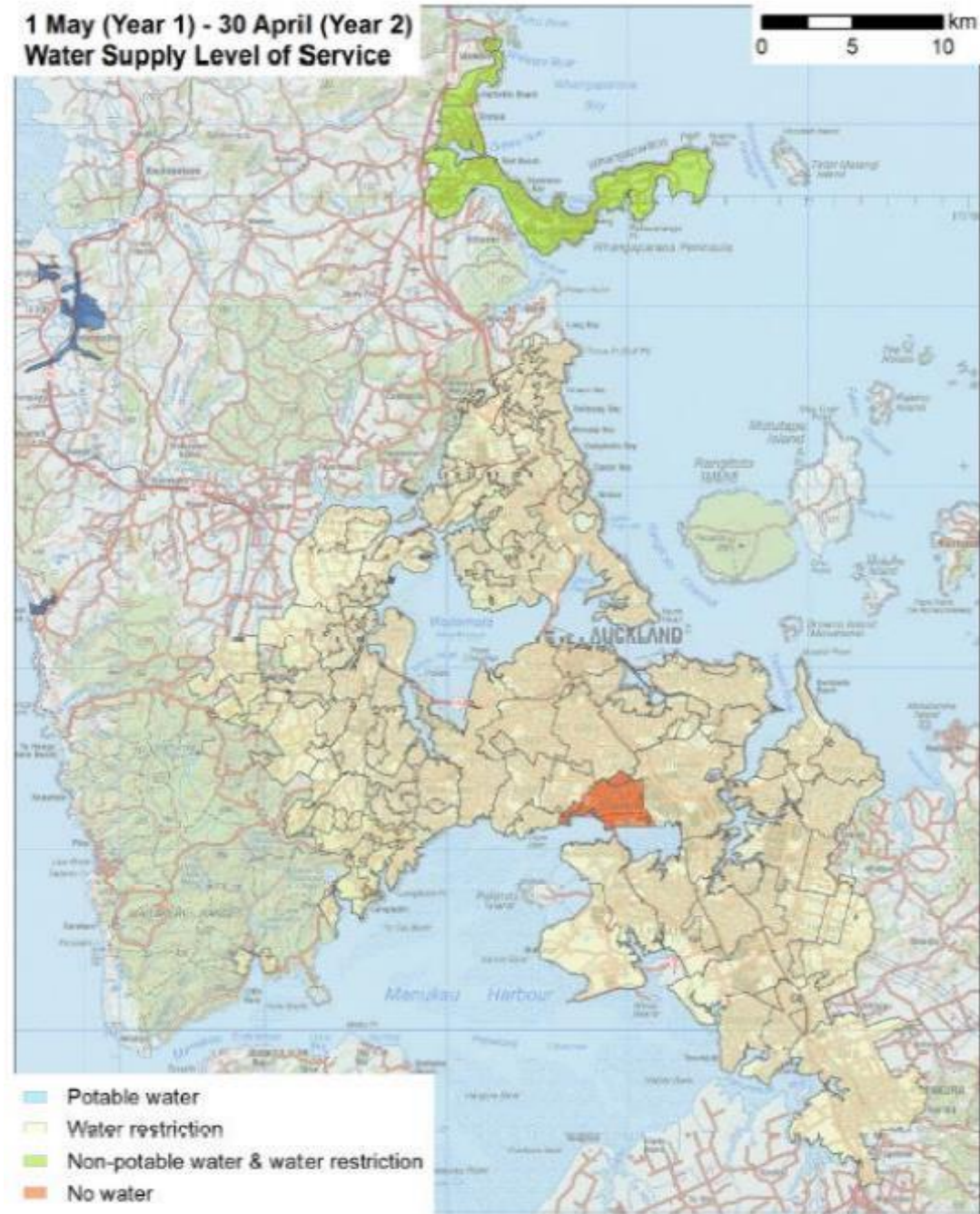
Figure 12.9 Water supply level of service map for period 1 May–30 April of Year 2. Water balance zones are colour coded according to service level, with blue for potable water, yellow for water restrictions, green for non-potable water and water restrictions, and red for no water.
