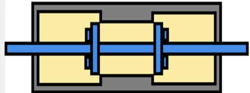
1-3 device has demonstrated potential to re-centre a structure with a residual drift (due to resistance away from centre)
