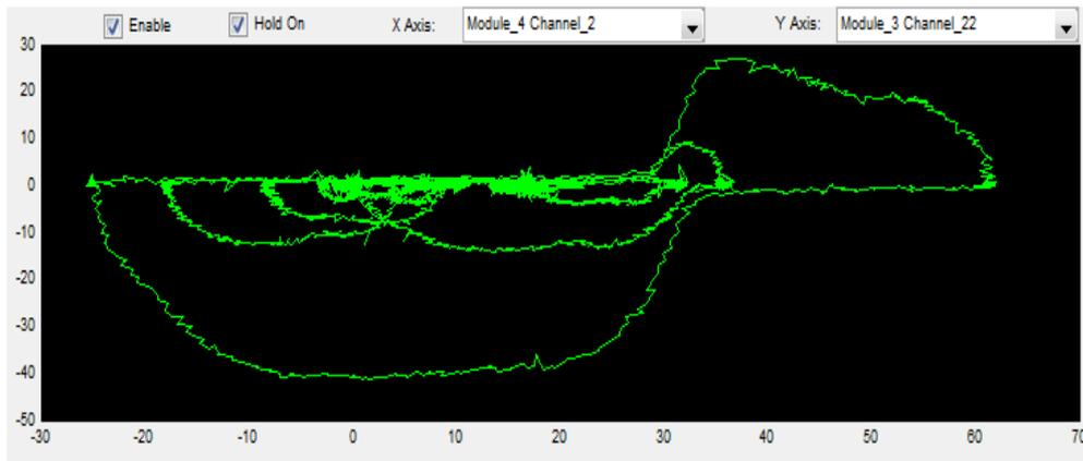
1-3 damping device as tested on the Auckland shake-table (the opposite diagonal to the 2-4 device)
