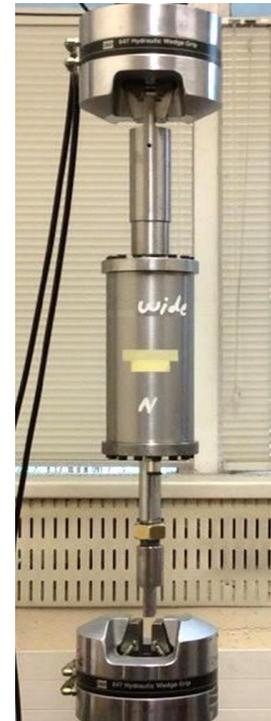
One way valves enables selection of when damping forces are provided to the structure, enabling the customisation of the overall hysteretic response.
