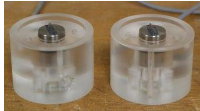
Bender elements and modified triaxial platens for V_p measurement
