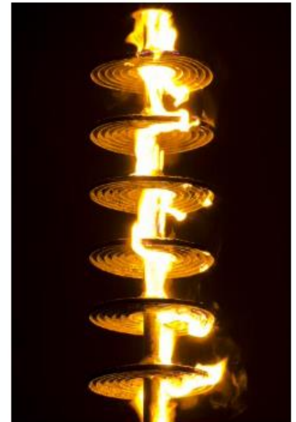
Flashover across composite insulator in lab (from Wardman et al., 2013)
