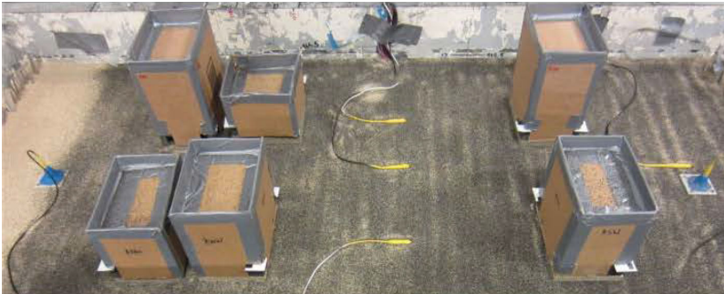
Geotechnical centrifuge test for studying SSSI on softened ground (Hayden et al., 2014)
