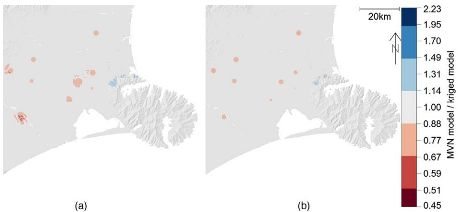
Figure 17. Covariance-adjusted MVN model V_{S30} predictions compared with RK predictions for (a) geology-based and (b) terrain-based models.
