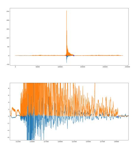
Other stations more difficult. Higher background noise means standard deviation trigger exceeded late, barely. "Quietens down" really fast after arrival. A higher high pass filter may be usefull.
