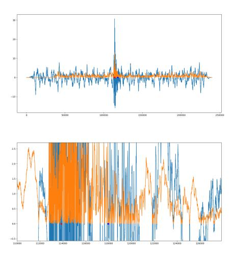
As background noise increases, it has a relatively lower frequency that dominates which means x intercepts at y=0 are fewer / unit time than during shaking.
