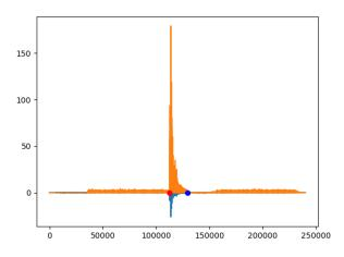
Able to pinpoint start of waveform by reversing until <3 standard deviations away from mean and then going further back until standard deviations from mean increases.
