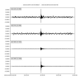
4th waveform looks clean. Standard deviations away from mean using a 3 minute window is below. Can use a 10 stdev trigger, making sure it goes higher once previous rolling window locked in place. Ends when standard deviation not exceeding 3 for 4 seconds.
