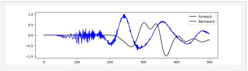
Backward wavefield using filtered adjoint source, high frequency noise generated flo=0.05 fmax=0.05 for seismogram filter
