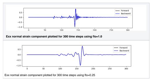
Comparision of adjoint sources with and without seismogram filtering
