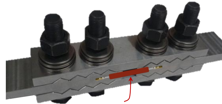
Displacement Sensor (e.g., potentiometer, LVDT/DVRT, portal gage) Could be powered by line or even self-powered (e.g., by disc piezoelectric generator)
