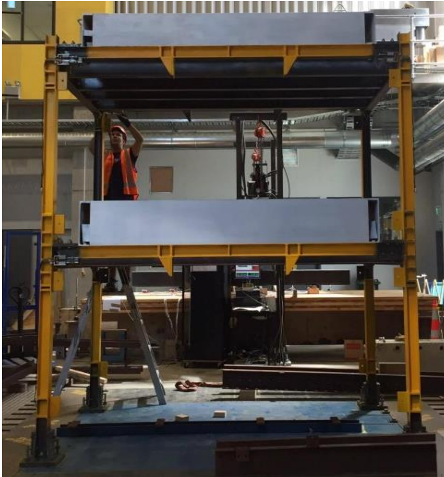
Large-Scale Testing (15 tonne structure) on the University of Auckland Shake-Table
