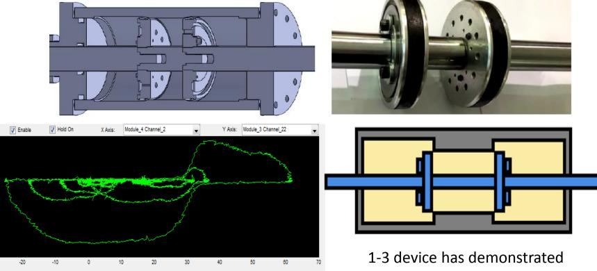
1-3 damping device as tested on the Auckland shake-table (the opposite diagonal to the 2-4 device) 1-3 device has demonstrated potential to re-centre a structure with a residual drift (due to resistance away from centre)
