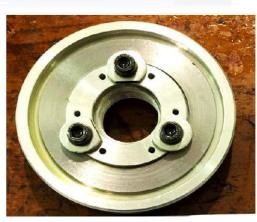
One way valves enables selection of when damping forces are provided to the structure, enabling the customisation of the overall structural hysteretic response.
