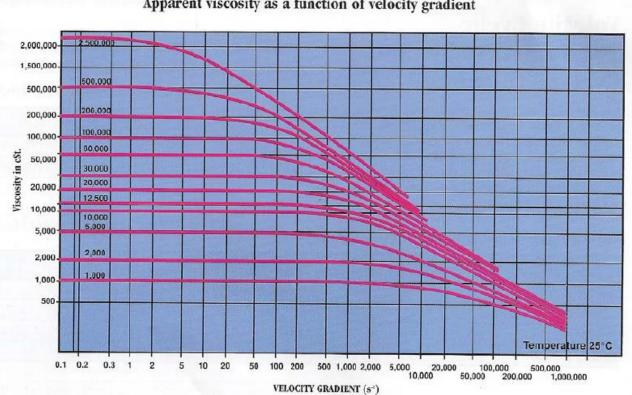
Apparent viscosity as a function of velocity gradient
