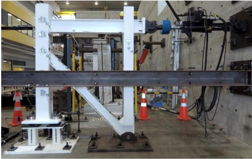
Bottom Storey RCBF Testing
