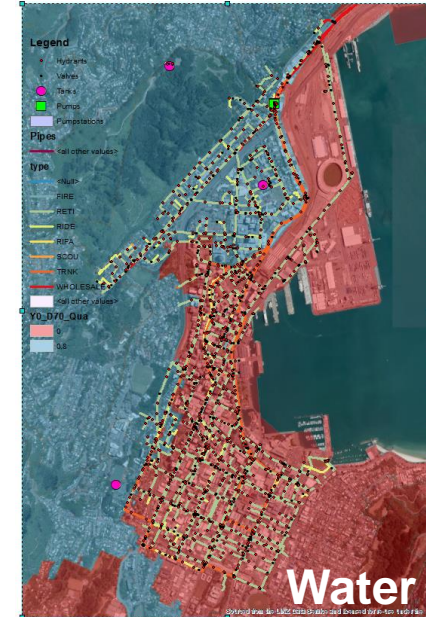
Damage to water networks
