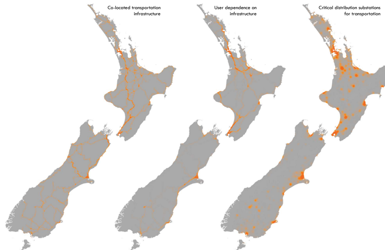
Fig. 2. National representations of co-located transportation infrastructures, the user dependence on transportation network components, and the dependence placed on distribution substations based on a quartic smoothing function.
