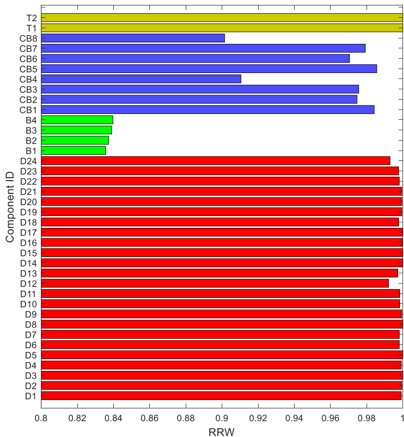
Figure 12 RRW of substation components in terms of ELNS (T: Transformer, CB: Circuit breaker, B: Bus bar, D: Disconnector)
