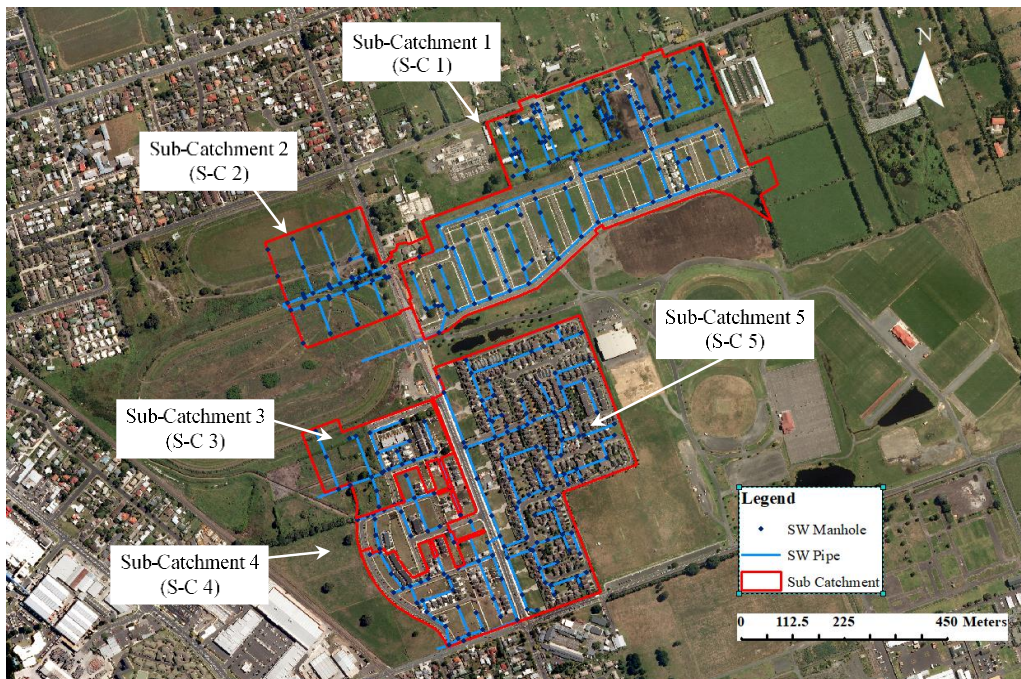
219 Figure 3: Plan of the stormwater network and sub-catchments of the study area.
